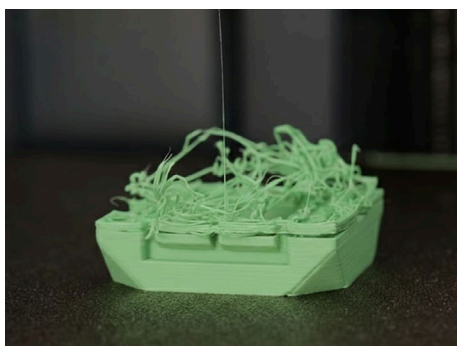
Air print, clogging, and under-extrusion
