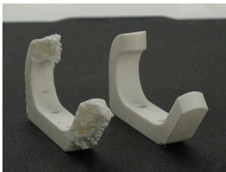
Poor overhang quality
