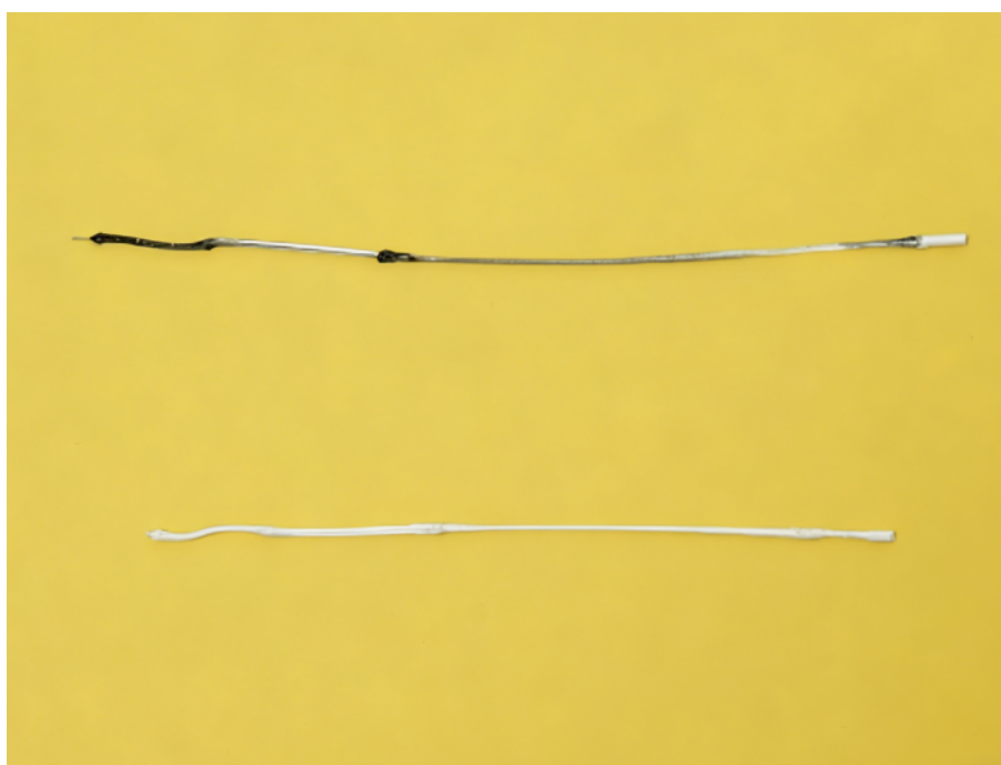
First cold pull (top) and after multiple cold pulls (bottom)
